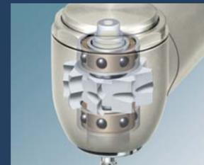
Because ceramic is 25% harder than stainless steel, it resists damage should debris enter the turbine. Ceramic is also 50% lighter in weight than stainless steel and therefore results in reduced friction with the bearing retainer. In combination, these factors are responsible for significantly extending bearing life.
