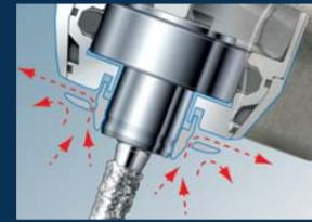
The NSK Clean Head System (Patented) is located in the handpiece head section. It is a special mechanism designed to prevent air retraction, and therefore the entry of oral fluids and other minute foreign substances into the turbine head.
