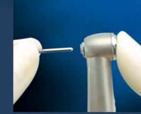
NSK triple grip Ultra Push Chuck (Patented) is an original design. The push button auto-chuck mechanism securely grips the bur during grinding conditions, and allows one-touch bur insertion and removal. The auto chuck lock mechanism is designed so that the bur retention capability increases when high load is applied to the bur.
